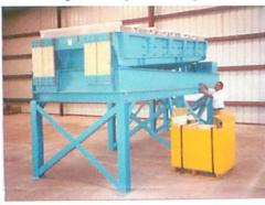
largest sized unit made. The large surface area of the roto shaker screens assures the product size is precisely controlled.
