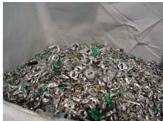
Figure 4: End caps separated by machine
