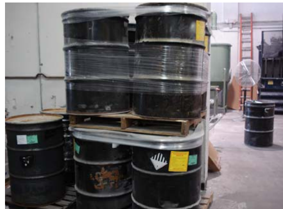
Figure 6: Phosphor powder hazardous waste drums
