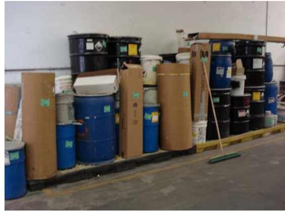
Figure 8: 90-day storage area
