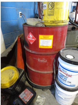
Figure 1. Hazardous Waste Label
