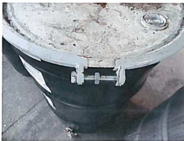
Figure 38: Nut and bolt closure on drum ring.
