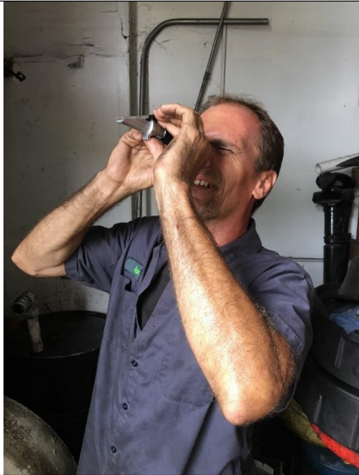
Photograph 2 – Fuels Unlimited employee checking the condition of recyclable coolant.
