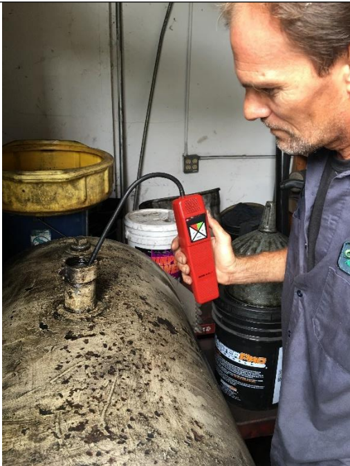
Photograph 3 – Fuels Unlimited employee using the M.T. Model TIFRX-1A "sniffer" at a customer's oil tank to screen for halogens before pumping to the collection tank truck.
