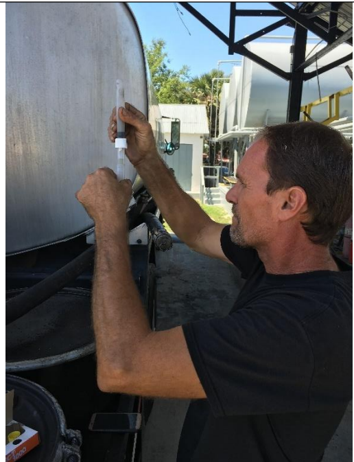
Photograph 4 – At the Fuels Unlimited facility checking halogen content of used oil using a Dexsil Chlor-D-Tect chlorine halogen test kit.
