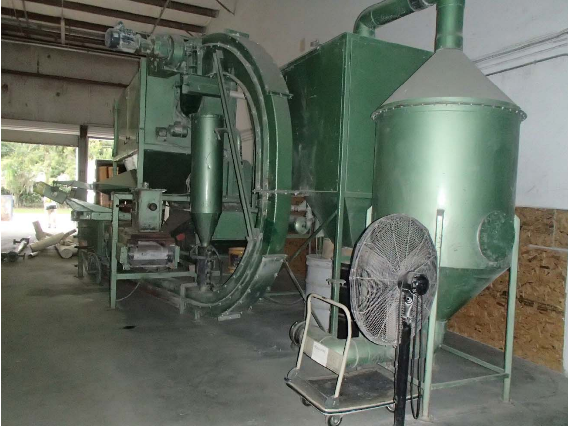
Figure 1. LSS1 lamp processor. The carbon silo is the tank in forefront of photo with the cone shaped extensions on top and bottom.
