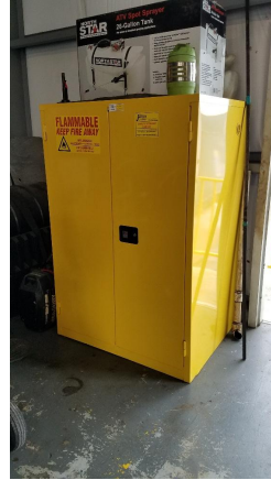
Flammable Storage Locker
