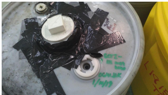
Improperly closed container
