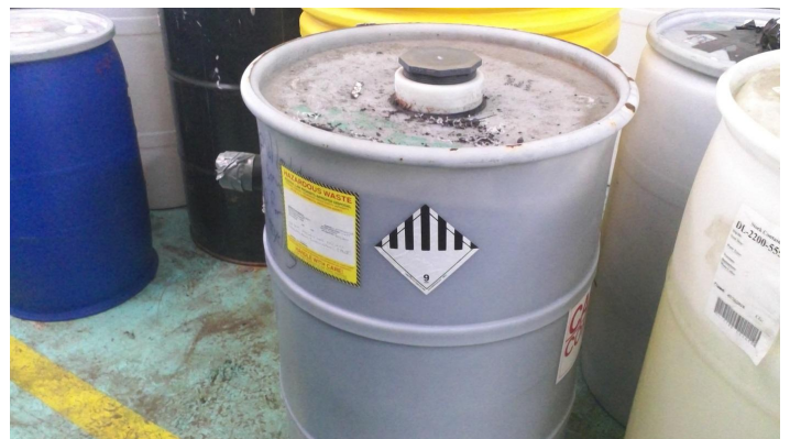
Improperly closed container
