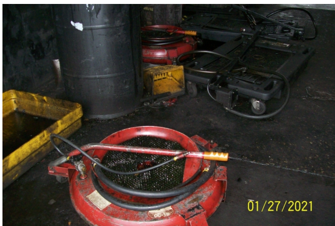
Unlabeled Used Oil Containers
