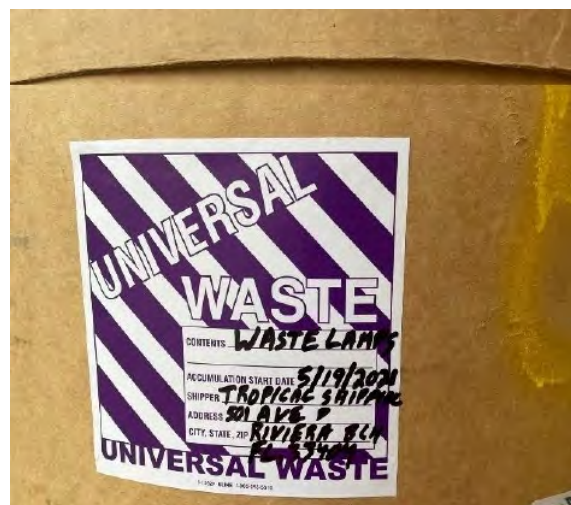
After - Properly Labeled Container with UW Lamps
