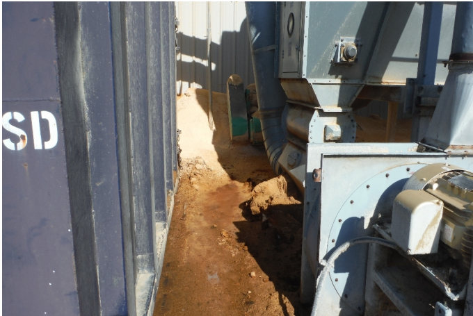
Photo 3 - Baghouse dust on concrete pad
