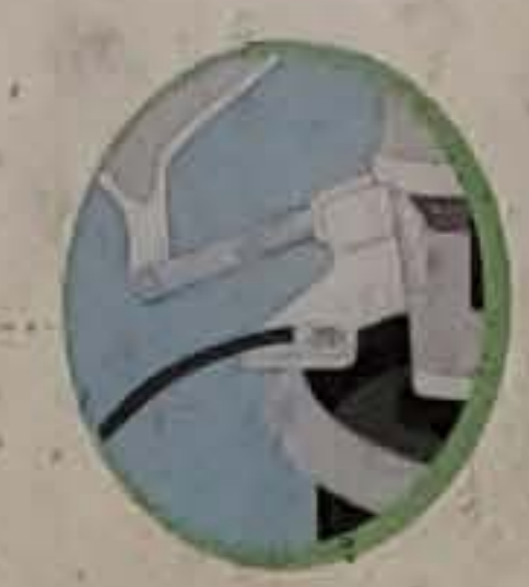
ANTI-STATIC WIRE Attach ring terminal of Anti-Static Wire to brass screw on Ground Support Plate of Puncturing Unit.
