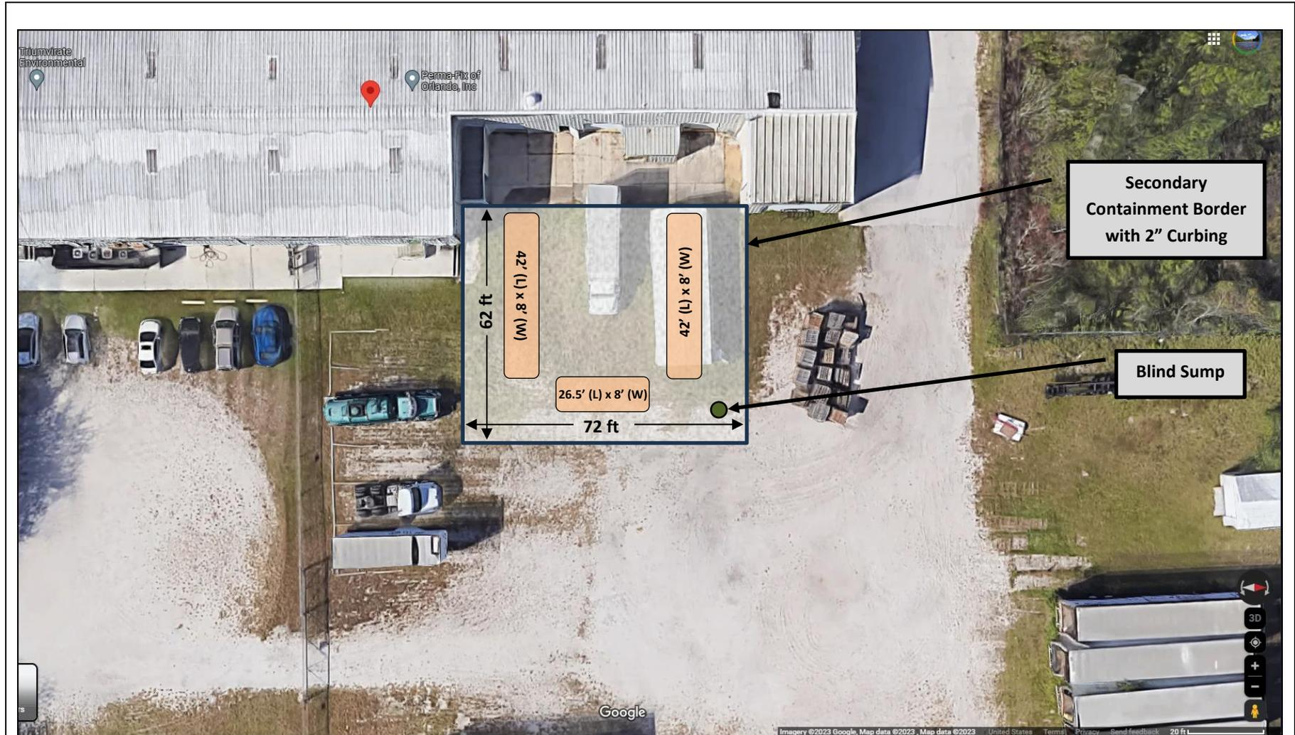
Total New Concrete Area Below Flammable Storage Units = 72 ft x 62 ft = 4,464 ft<sup>2</sup> (with a 2" curb around the perimeter)
