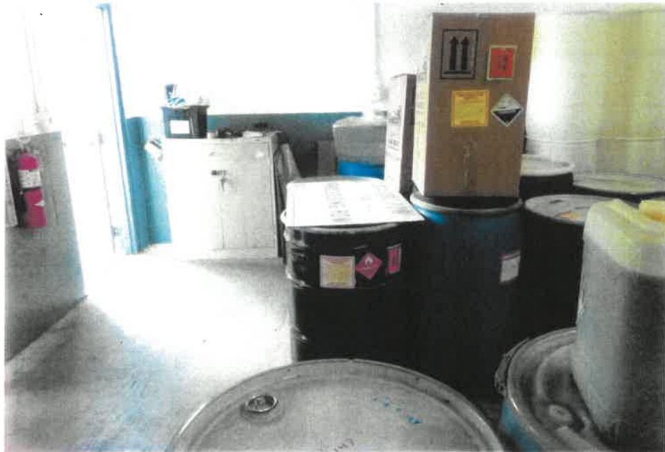
Photograph 13: Two 55-gallon containers of flammable hazardous waste in the staging area of Bay 3, that within 50 ft. of the north property boundary Photo taken by Javier García, on 6/20/2018, at 12:16 p.m. Equipment used: Samsung Camera (Model WB250F)-EPA Property Tag # S75951
