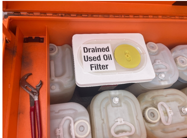
Corrected: Labeled Used Oil Filter Container
