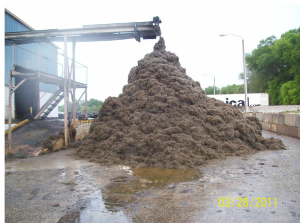
Steel fiber residue.
