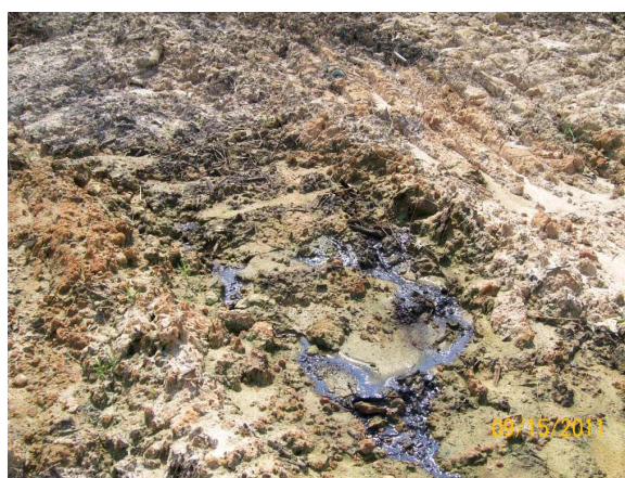
Phase 2 leachate seep
