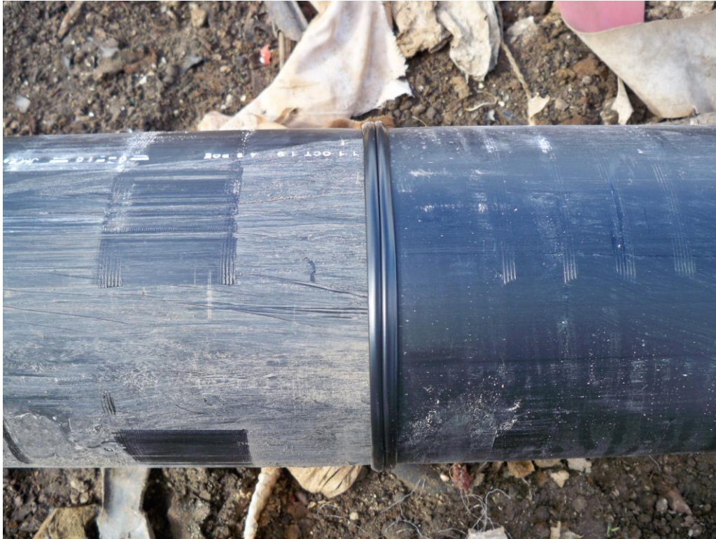
Photograph 19: HDPE SDR 17 hard weld showing acceptable bead.
