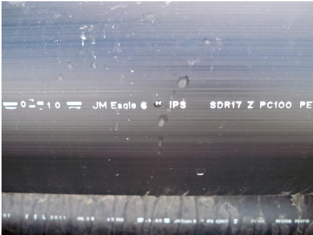
Photograph 15: 6" HDPE SDR 17 pipe.
