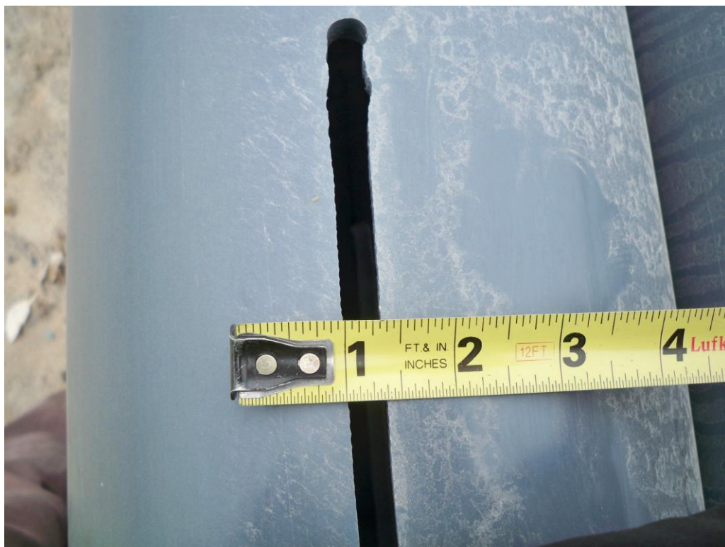
Photograph 10: 8" SCH 80 PVC slot width.
