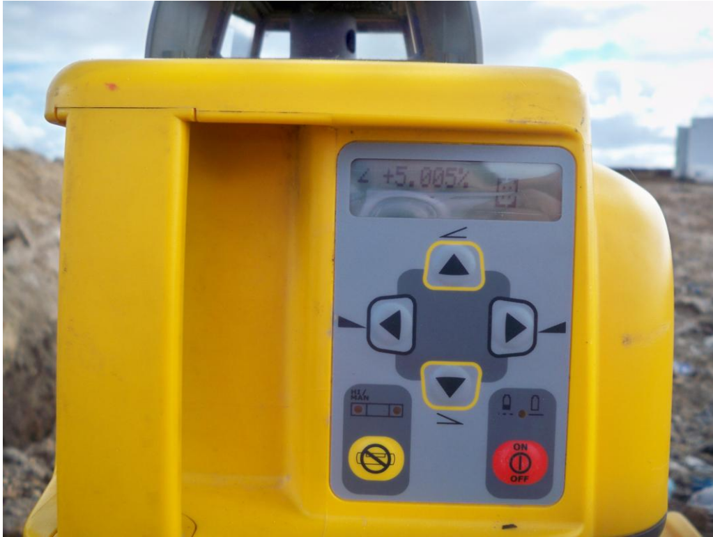
Photograph 23: Survey slope construction laser set at 5% for trenching laterals and header (typical).
