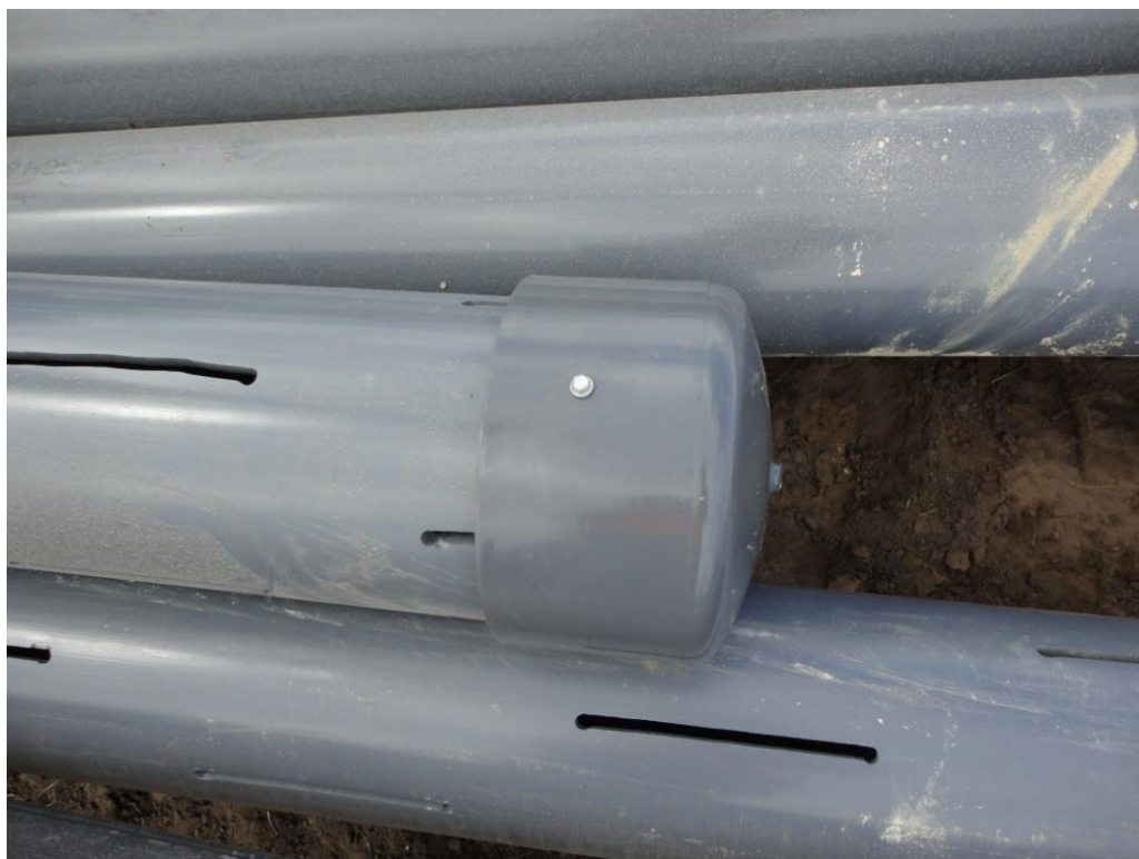
Photograph 14: 8" SCH 80 PVC cap with lag bolts.
