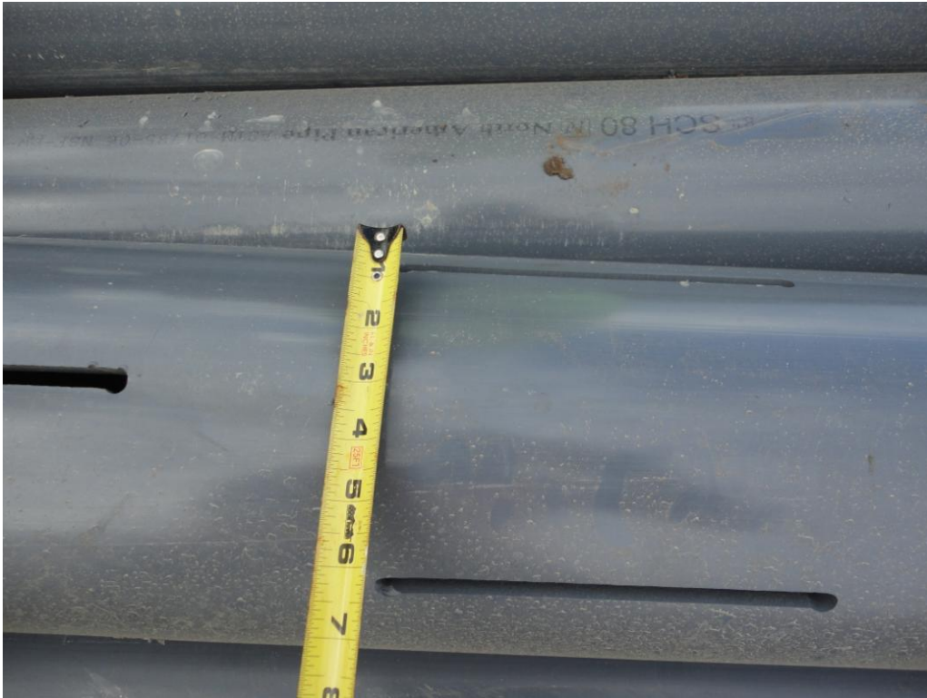
Photograph 11: 8" SCH 80 PVC 45° apart, staggered rows.
