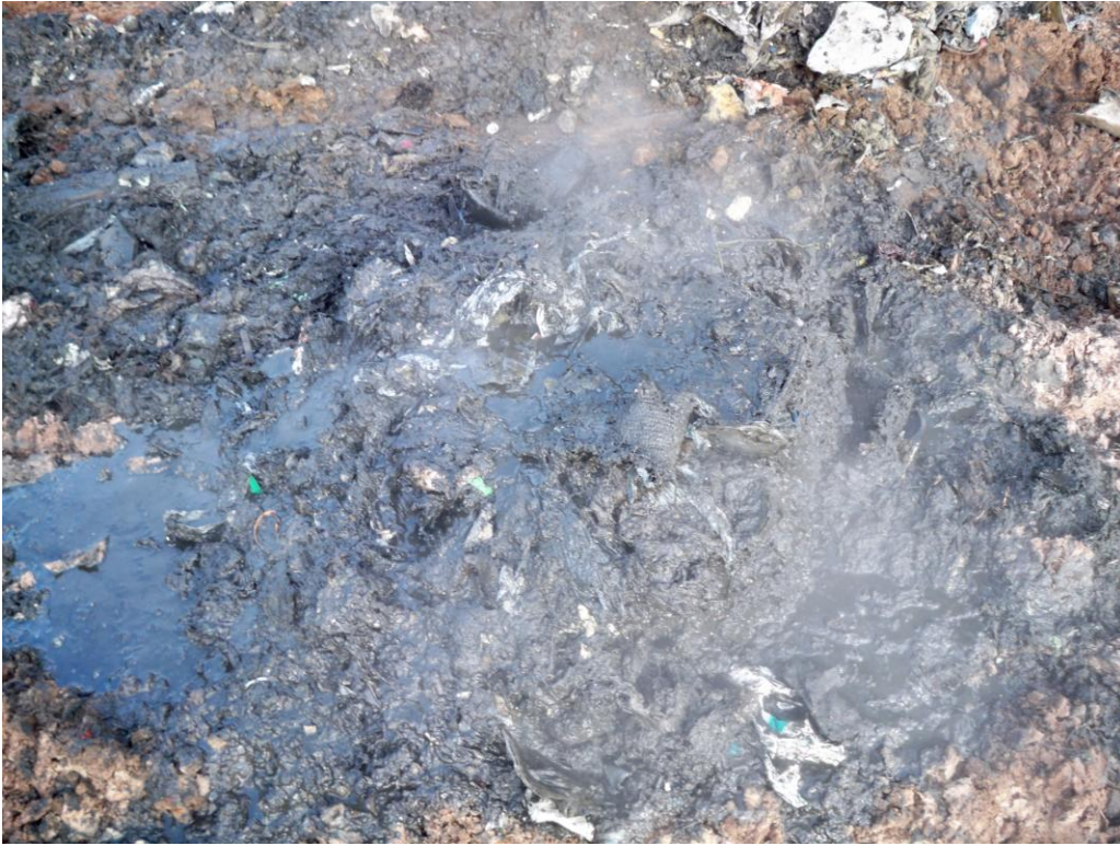
Photograph 39: Encountered saturated materials that could not be excavated using a bucket auger (typ).
