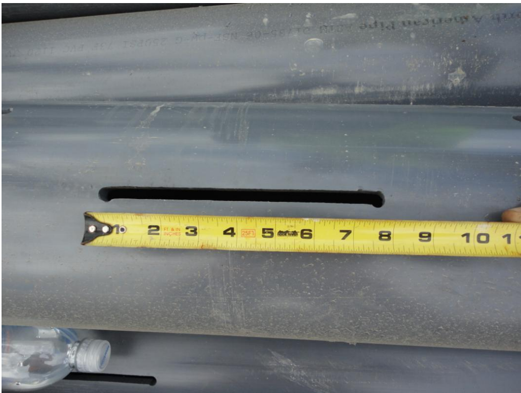
Photograph 12: 8" SCH 80 PVC slot length.
