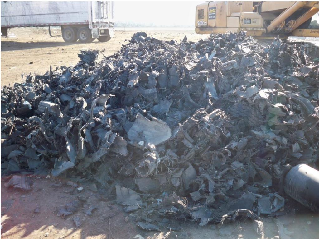
Photograph 48: Tire chips used for HGC backfill (typical).
