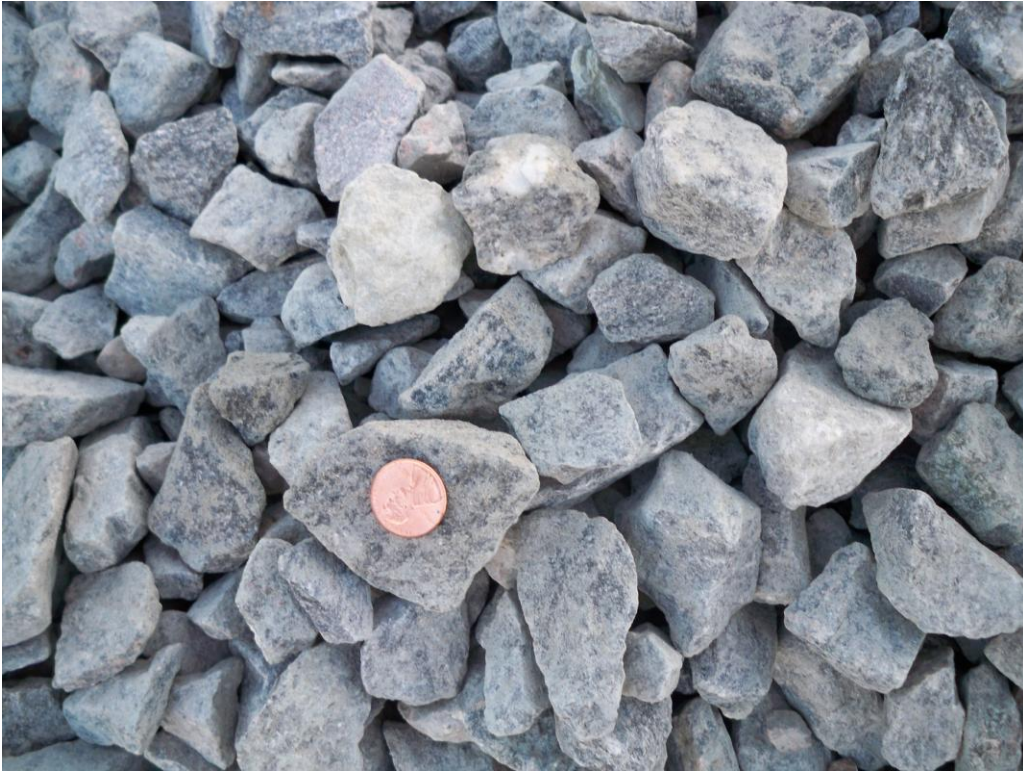
Photograph 7: Gravel backfill for extraction wells. Lab analysis: gravel finer than No. 4 sieve is 0.2%, gravel finer than No. 200 sieve is 0.1%, carbonate content is 0.1%.
