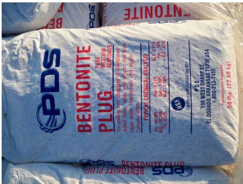
Photograph 35: Bentonite used for plugs at extraction wells.
