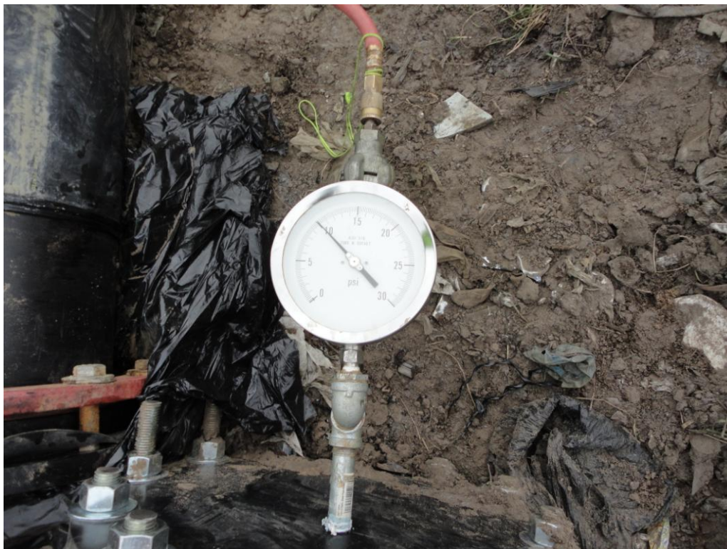
Photograph 20: Air testing 12" HDPE SDR 17 header in Cell 5 (passed).
