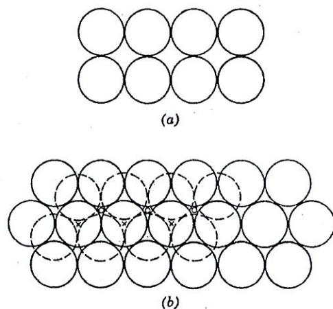
Fig. 3.2 Arrangements of uniform spheres. (a) Plan and elevation view: simple cubic packing. (b) Plan view: dense packing. Solid circles, first layer; dashed circles, second layer;  $\circ$ , location of sphere centers in third layer; face-centered cubic array;  $\times$ , location of sphere centers in third layer: close-packed hexagonal array. (From Deresiewicz, 1958.)
