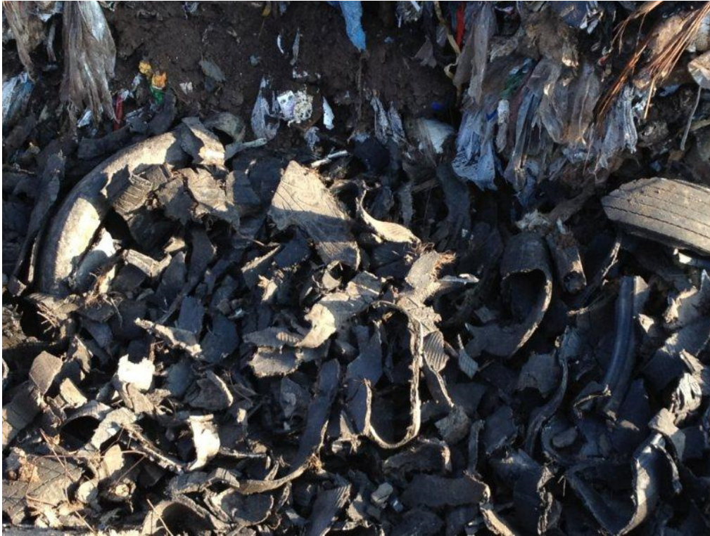
Photograph 49: Tire chips used for drainage fill in HGC trenches (typical).
