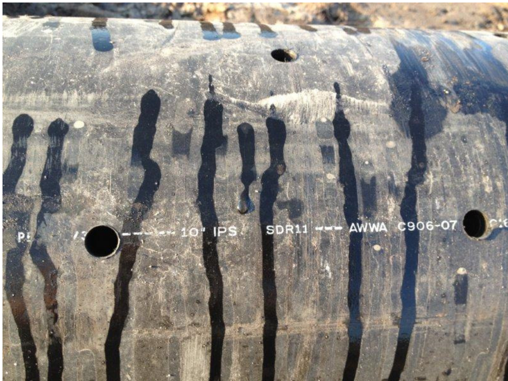
Photograph 46: 10" HDPE SDR 11 pipe for HGC's.
