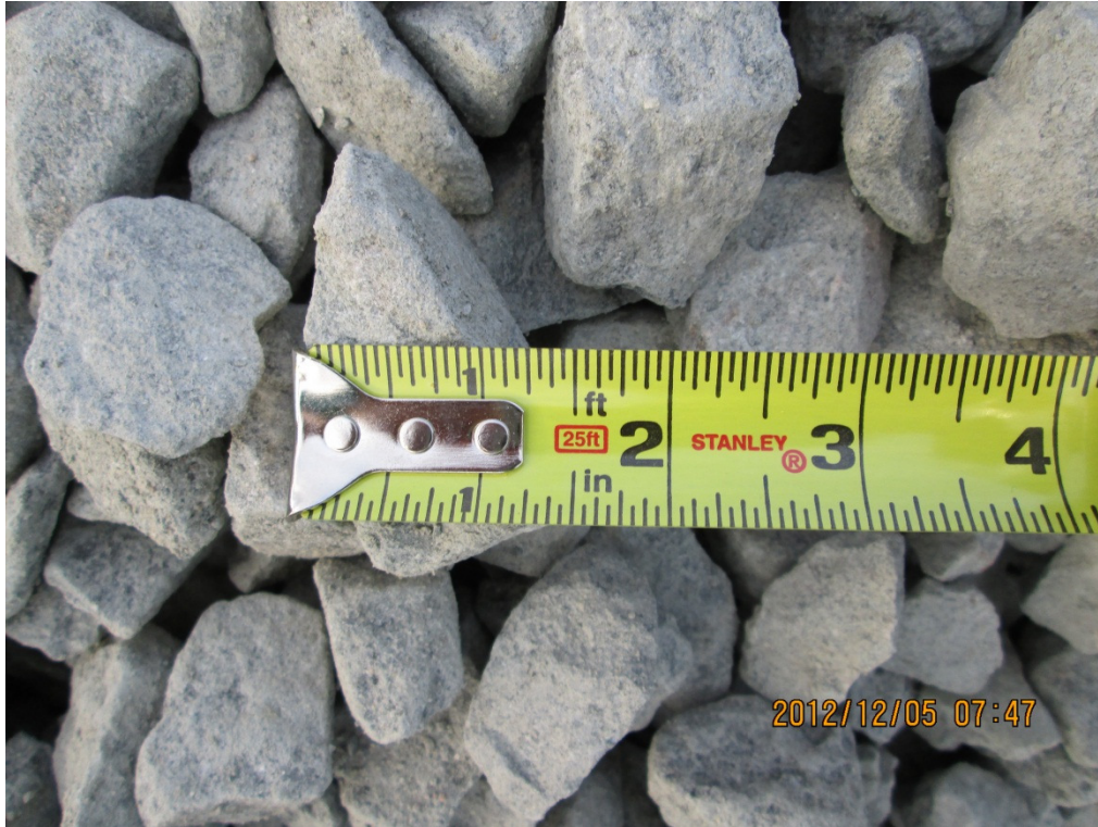
Photograph 1: Gravel backfill for extraction wells. Lab analysis: gravel finer than \frac{3}{4} " sieve is 6.2%, gravel finer than No. 4 sieve is 1.2%, gravel finer than No. 200 sieve is 0.2%, carbonate content is 0.1%.
