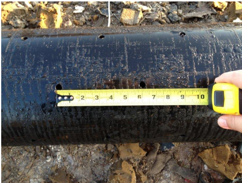
Photograph 47: 10" HDPE SDR 11 perforation sizing and spacing.
