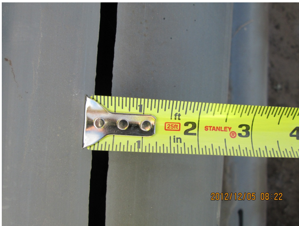
Photograph 4: 8 inch SCH 80 PVC slot width.
