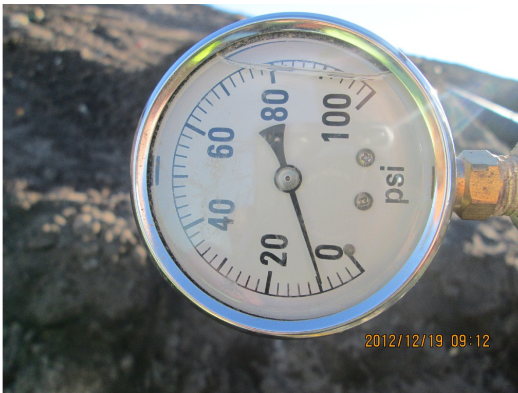
Photograph 12: Air testing gas conveyance system in Cell 8 (passed).
