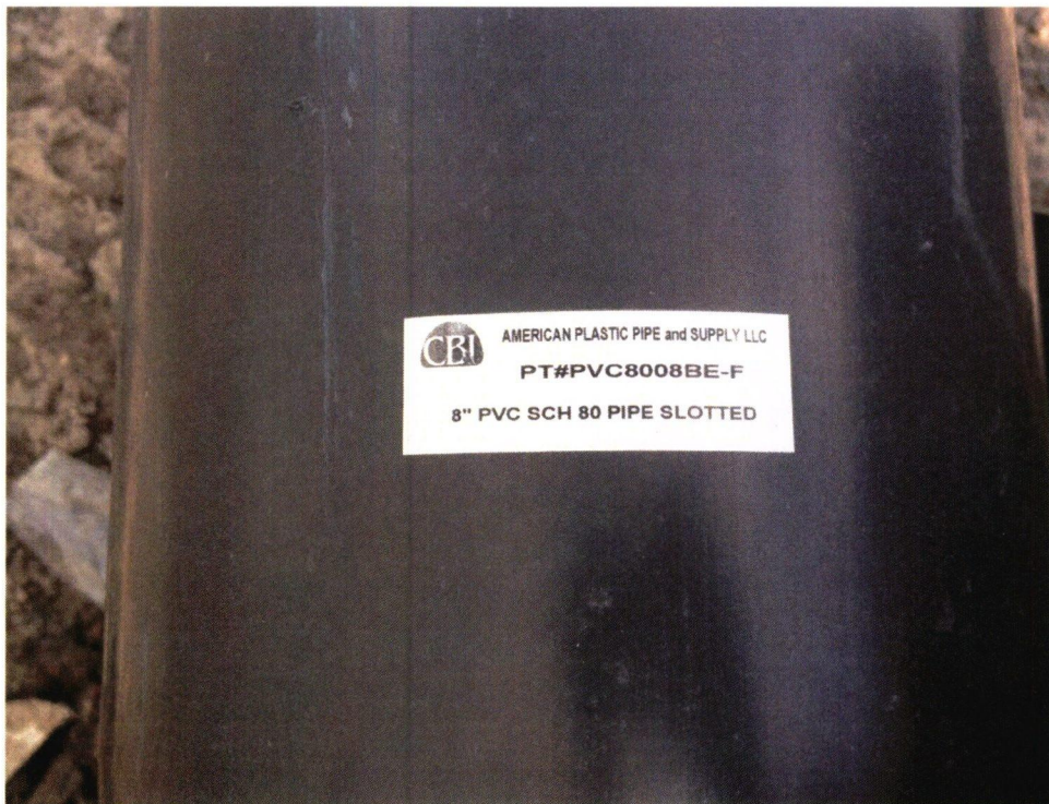
Photograph 2: 8" SCH 80 slotted PVC pipe.
