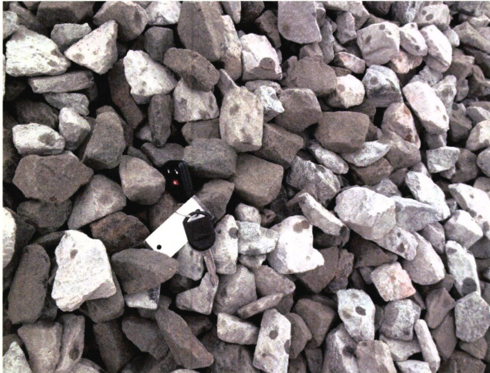
Photograph 1: Gravel backfill for extraction wells. Lab analysis: gravel finer than 3/4" sieve is 1.4%, gravel finer than No. 4 sieve is 0.7%, gravel finer than No. 200 sieve is 0.2%, carbonate content is 0.1%.
