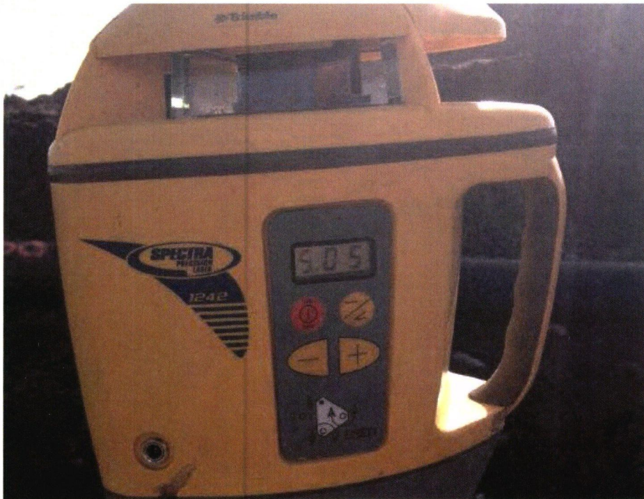
Photograph 37: Slope setting for CB&I laser level.
