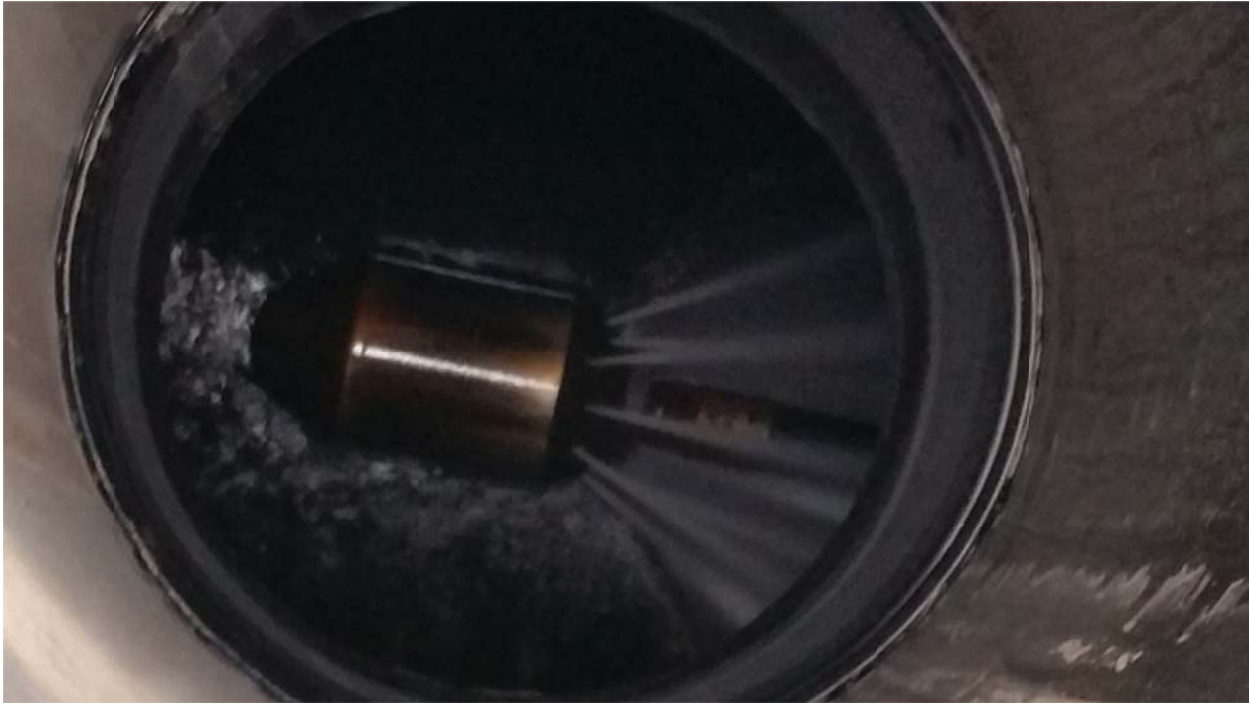
Spray Nozzle of Water Pressure Jet Cleaning
