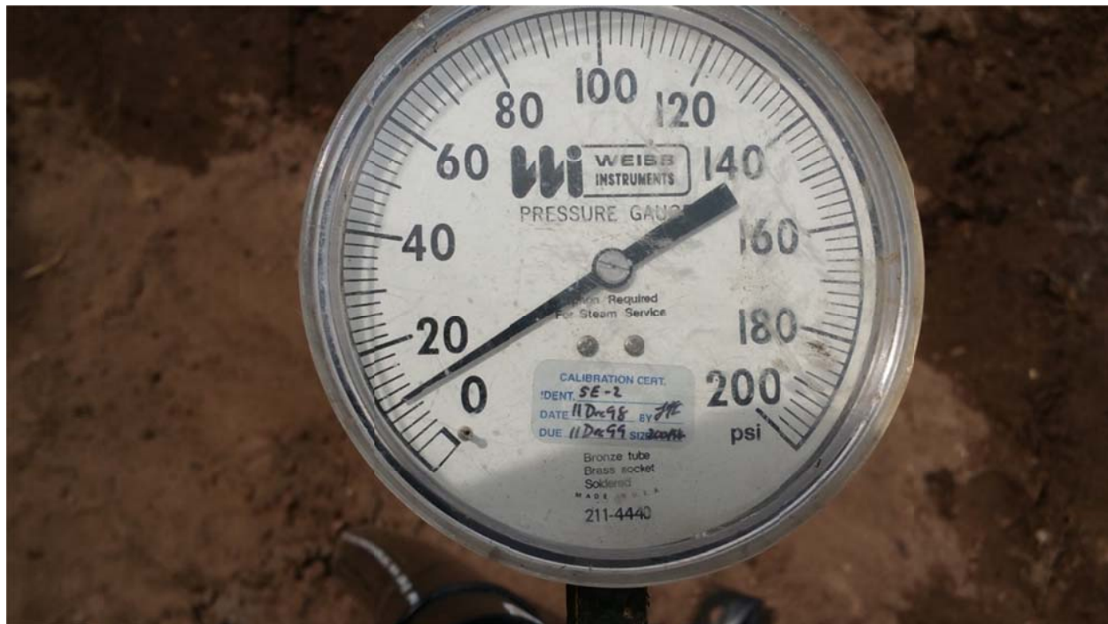
Pneumatic Pressure Test of Air Line (Maintain 10 psi)
