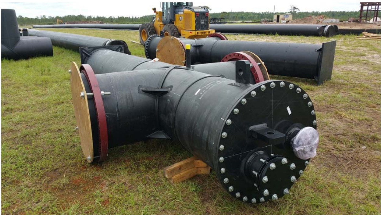
Pre-fabricated Condensate Sumps
