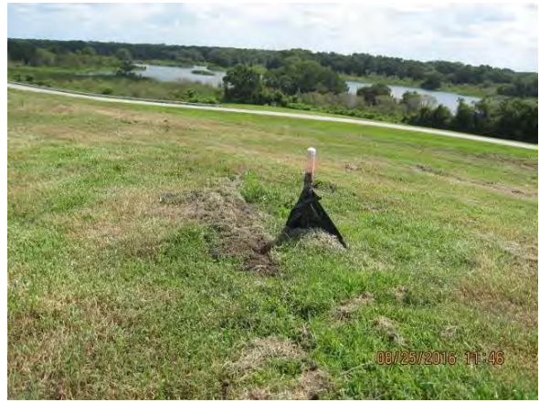
Phase II Piezometer
