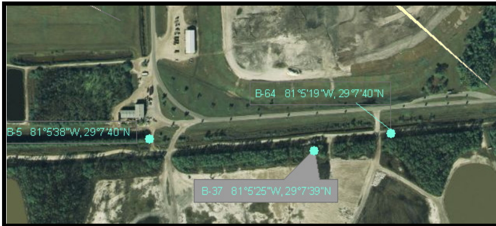
Figure A--MW locations plotted by GIS from survey table of latitude and longitude submitted 12/07.
