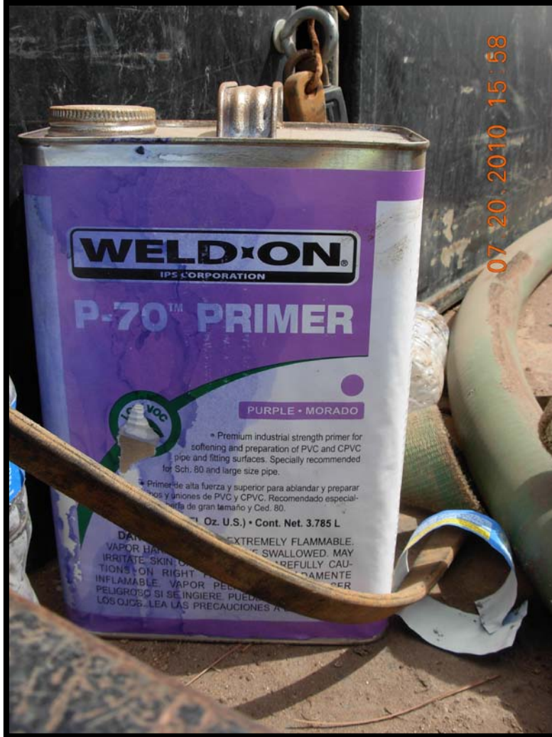
Photograph 46: PVC primer used prior to PVC cement when joining well casing joints.
