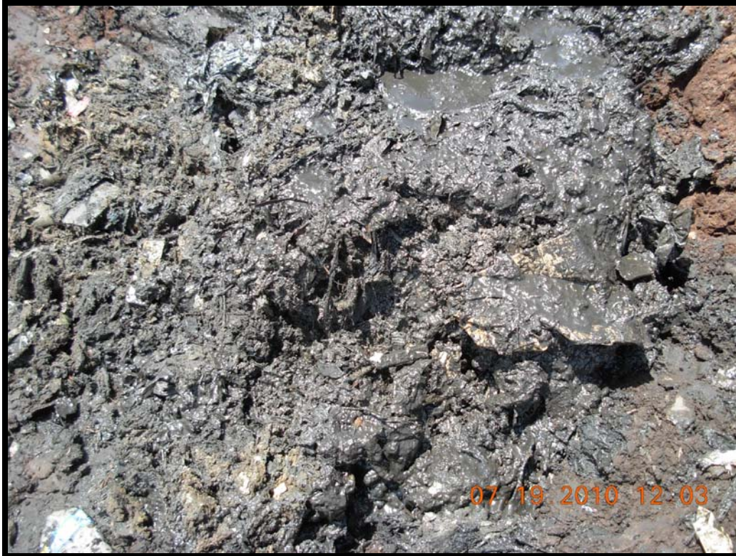
Photograph 44: Encountered saturated materials that could not be excavated using a bucket auger at GW-54.
