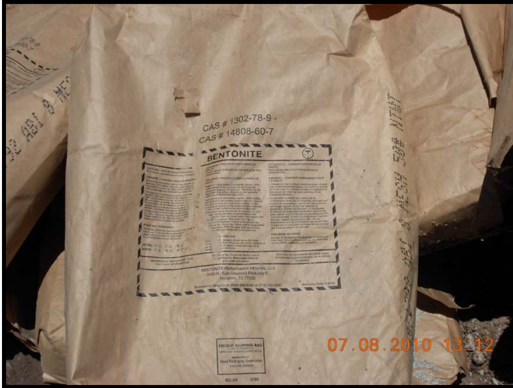
Photograph 21: Bentonite used for plugs at extraction wells.
