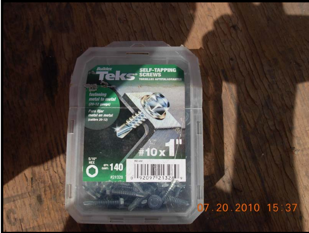
Photograph 47: Self tapping screws used to supply additional support at each well casing joint.
