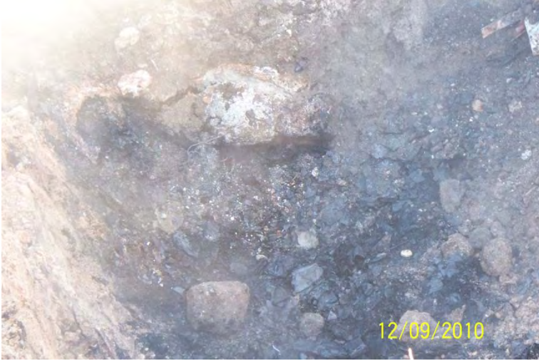
12/9/2010 Charred and burnt waste and ash in excavation 100_0579.JPG
